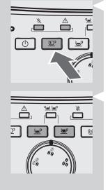
2 Press the "D" button to start the cycle. The machine starts the automatic priming of the circuit by dispensing some water through the Pannarello.
