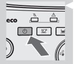
1 Turn off the machine by pressing the "()" button and remove the plug from the socket.
