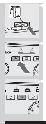
12 Switch the power button located on the back of on the machine to "I".
