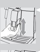
The height of the dispensing spout can be adjusted to better fit the dimensions of the cups that you wish to use.
