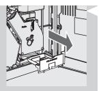
3 Empty and clean the coffee residues drawer located in side of the machine. Open the service door, remove the drawer and empty the coffee residues.
