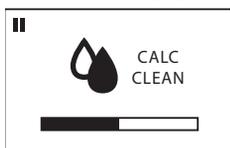
You can pause the descaling or rinsing cycle by pressing the ESC button. The display will show the following icon. To continue the descaling or rinsing cycle, press the OK button.
