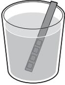
To be able to adjust the machine settings to the water in your region, please measure the water hardness with the water hardness strip supplied.
