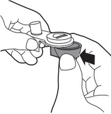
**16** Attach the automatic milk frother to the fitting and make sure it is locked into place.
