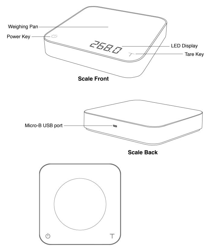
\*Note: For the best performance, place the weight in center of weighing platform.
