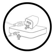
• To use AC adapter instead of the built-in battery, plug the USB cable into the Micro-B USB port located on the back panel of the scale.
