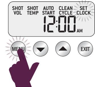
Press UP or DOWN arrow to adjust the time. For faster scrolling, press and hold the UP or DOWN arrow. Press the EXIT button to set.
