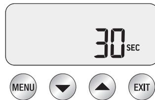
Shot clock will be displayed during an extraction and 10 seconds after the extraction before returning to the default shot temperature display mode.
