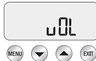
Select between volume based (FLo) or time based (SEc) method for espresso dose measurement. While 'vOL' is displayed on the LCD, press MENU button. Press UP or DOWN arrow to the desired method. Press MENU button to set. Machine will beep to confirm selection.
