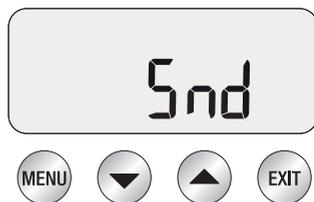
Adjust the audible alerts. While 'Snd' is displayed on the LCD, press MENU button. Press UP or DOWN arrow to off (OFF), low (LO) or high (HI). Press MENU button to set. Depending on the selected setting, the machine may beep to confirm selection.
