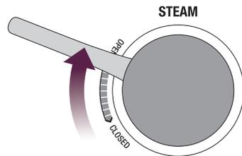
To turn steam off, move STEAM LEVER to CLOSED position. The machine will return to STANDBY mode.
