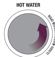
To turn hot water off, rotate the HOT WATER dial to CLOSED position. The machine will return to STANDBY mode.
