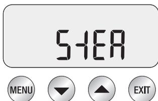
Adjust the steam boiler temperature, which in turn controls steam pressure. Lower steam temperature to texture smaller volumes of milk or to have more control. Increase steam temperature to texture larger volumes of milk. While 'StEA' is displayed on the LCD, press MENU button. Press UP or DOWN arrow to the desired temperature. Press MENU button to set. Machine will beep to confirm selection.
