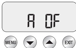
Use this function to disable the Auto Off feature. While 'A OF' is displayed on the LCD, press MENU button. Press UP or DOWN arrow to select off or on. Press MENU button to set. Machine will beep to confirm selection.
