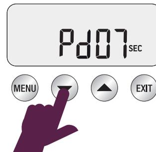
We recommend a range between 5-15 secs as being optimum. Press MENU button to access Pre-Infusion Power, or press EXIT button to set.
