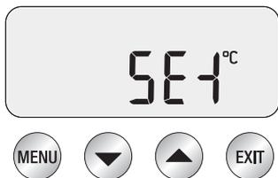
Set units to metric or imperial. While 'SEt' is displayed on the LCD, press MENU button. Press UP or DOWN arrow to the desired unit. Press MENU button to set. Machine will beep to confirm selection.
