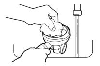
The filterholder should be cleaned to remove the greasy coffee residues that can negatively affect the taste of your espresso. Wash the exterior part of the steam wand with a damp cloth and release a little steam to remove any milk residues from inside the tube, as these could obstruct the steam output, making it more difficult to froth milk properly.
