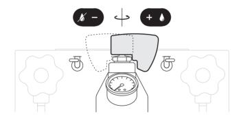
**C.3** Once the display shows the icon of the lever upwards, move the lever (13) completely up.
