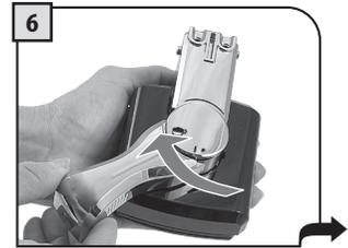
6 Rotate the handle clockwise up to the ☕ symbol.
