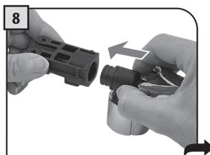
8 Remove the external fitting by pulling it.
