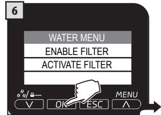
Access the "MACHINE MENU" (see page 25). Select "WATER MENU" and "ACTIVATE FILTER", then press "OK".
