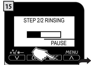
If the containers need to be emptied, press the "PAUSE" button. Then, press the "START" button when the container has been emptied and replaced.
