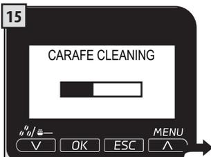
The cleaning cycle is activated. The bar shows the cycle progress.
