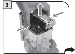
3 Press the disengage buttons to allow the lid removal.
