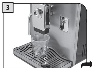
**Note:** In some cases the dispensing spout can be removed to allow the use of very large containers.
