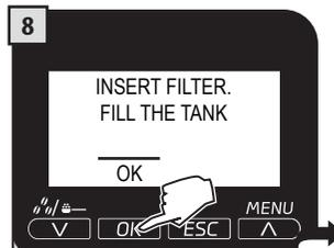
Press the "OK" button to confirm the introduction of the new water filter.
