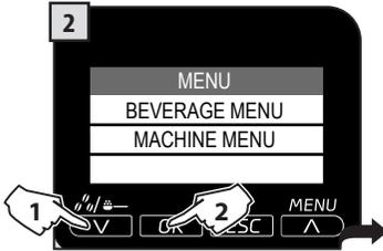
Select the menu by pressing the (V) button. Press the OK button to access the MACHINE MENU.
