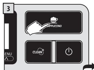
3 Hold the button pressed for 3 seconds to start programming.
