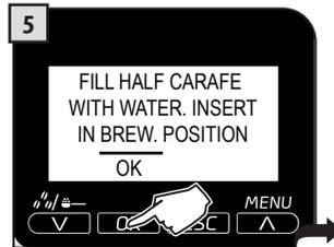
Fill half the carafe with fresh water (page 34 - fig. 7). Insert the carafe and place it in the brewing position. Then, press the "OK" button.
