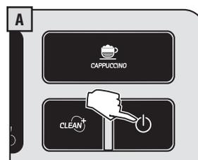
The red light flashes when the machine is in stand-by mode.
