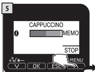
5 Milk dispensing begins. When the desired quantity has been reached, press "STOP".
