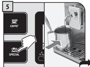
5 At the end of the dispensing phase, remove the container and place it under the hot water wand. Press the "SPECIAL" button.
