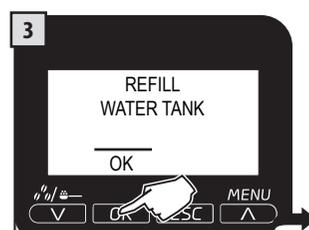
Fill the water tank with fresh drinking water. Press the "OK" button to confirm.
