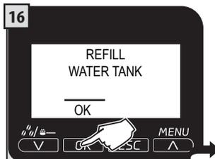
At the end of the wash, fill the tank with fresh drinking water. Press the "OK" button to confirm.
