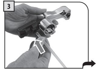
3 Insert the hose in the outer fitting.
