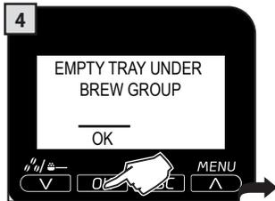
Empty the drip tray placed under the dispensing spout (page 36 - fig. 2) and then replace it on the machine. Then, press the "OK" button.
