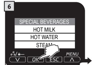
6 Select "HOT WATER" by pressing button (∧) or (∨). Press the "OK" button and wait for the programmed quantity to be dispensed.
