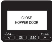
Close or correctly place the coffee bean hopper inner cover to be able to prepare a beverage.
