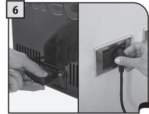
Insert the plug into the socket located on the back of the machine and insert the other end into a power outlet with suitable current.
