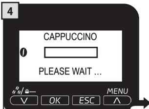
4 The machine starts brewing: it grinds the coffee and warms up to dispense milk. In this case the ECOMODE function is set to "ON" (see page 26).
