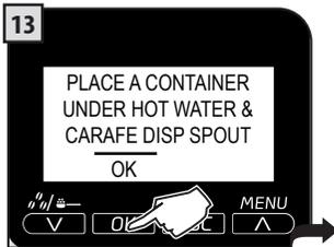
Place a container under the dispensing spout and a container under the hot water wand. Then, press the "OK" button.
