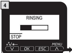
When warm-up phase is complete, the machine performs a rinsing cycle of the internal circuits. It is possible to interrupt the cycle by pressing the "STOP" button.
