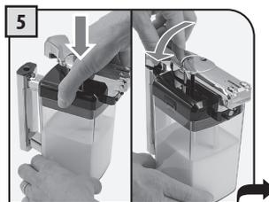
5 Place the lid back and ensure that it is closed correctly. Move the handle back to its central position to allow for perfect closure.
