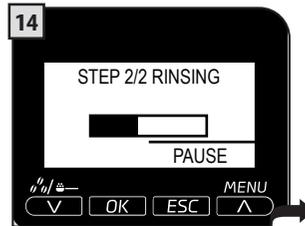
The rinse cycle is activated. The bar shows the cycle progress.
