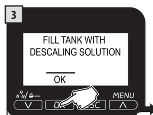
Refill water tank with descaling solution.
