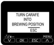
A beverage with milk has been selected. The machine requires the carafe handle spout to be placed into dispensing position.
