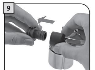
9 Remove the internal fitting.
