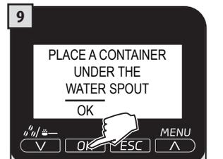
Press the "OK" button to confirm. Wait until the cycle is completed and remove the container.
