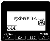
The machine requests the "Intenza" water filter to be replaced with a new one. Replace the filter as described on page 7.
