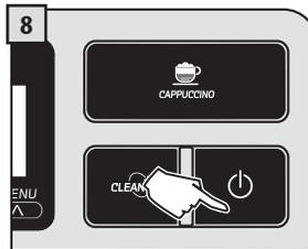
The display shows a red flashing led. Press the stand-by button to start the machine.
