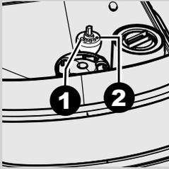
The reference marks inside the coffee bean hopper indicate the grind setting. There are 5 different grind settings to choose from with the following references:
