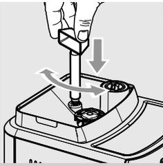
Press and turn the pin one notch at a time and brew 2-3 cups of coffee; this is the only way to notice differences in grind.
