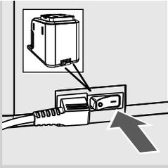
**9** Switch the power button to "I" to turn on the machine.
