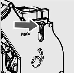
**8** Make sure the hook to lock the Brew Group is in the correct position; to check its position firmly press the "PUSH" button.
