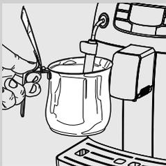
In order to avoid that any water is left in the circuit for a long time, before starting the machine for the first time, and after long periods of inactivity, the water circuit needs to be primed. This is because we want to offer you a perfect and fresh product.
