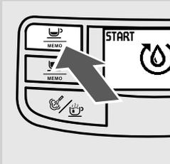
**2** Select "START" by pressing the "☺" button. The machine starts the automatic priming of the circuit by letting out a pre-set quantity of water through the Pannarello. The bar under the icon shows the operation progress.
