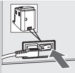
**12** Switch the power button located on the back of on the machine to "I".
