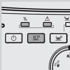
**14** The "⚠" and "⚠" lights and the "⏻" button light will begin to flash quickly indicating that the water circuit must be primed.
