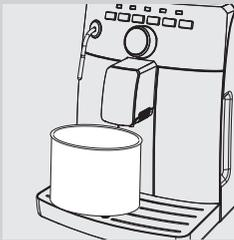
**10** Remove the water tank, rinse it and fill it up to the MAX level with fresh water. Place it back into the machine.
