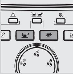
4 The machine warms-up and the “☕” “☕” buttons flash. The “✎” button turns off.
