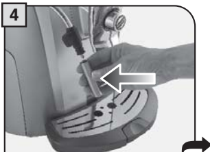
Remove the outer sleeve of the hot water/steam wand; thoroughly rinse it under running water, then re-insert it.
