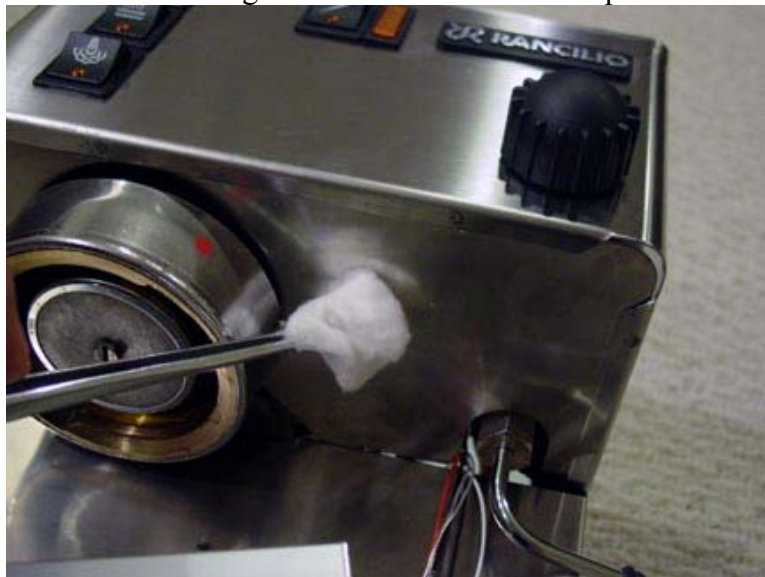
Figure 22. cleaning the box mounting area with alcohol.
