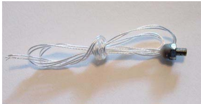
Figure 6, Temperature sensor (Pt100 RTD) with screw tip.
